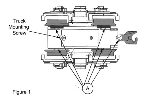
1. For the axles and coupler pivot points **Marked A**, we recommend that you lubricate with a small amount of light oil such as Bachmann E-Z Lube® #99984 Light Gear Oil. **Do not over-lubricate**.
